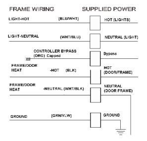
Figure 4 Wiring W/O Energy Controller
