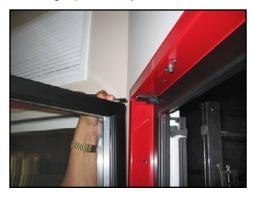
6. Lift the door out of the torquemaster. Secure or lean the door on its side against a stable surface.
