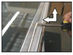
12. Manually pull out and remove the remaining heater wire.
