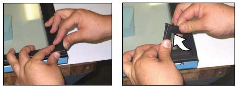
2. Carefully pull the gasket out of the grove in the plastic rail covers.
