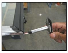
4. Upon replacing the hinge pin, insert all three wires into the hinge pin hole in the door rail.
