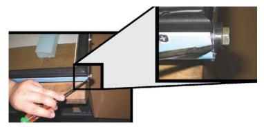
2. Dislodge the torque rod from its mount by pushing on the torque rod or tap it loose using a plastic or rubber mallet.
