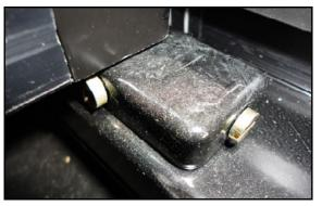
Insert Torque Rod into Torquemaster
