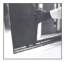
3. If optional spring closers are in place, unhook spring from hook on top of door before removing door.
