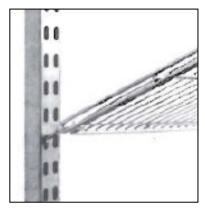
7. Drop rear of shelf down and pull back in slot on rear posts. Continue to add shelves behind each door, spacing for desired product merchandising.
