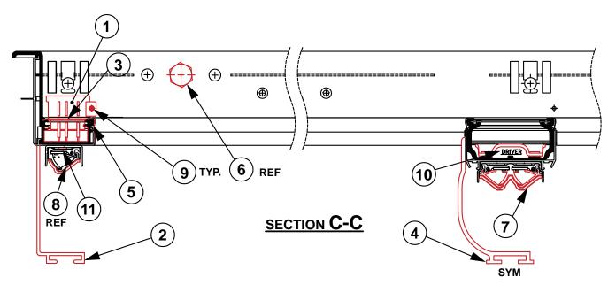
Model 401 Frame Section C Replaceable Parts
