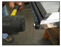
2. To remove, lay a flat-head screwdriver parallel to hinge rail, catch edge of bottom of torque rod shaft and tap out.
