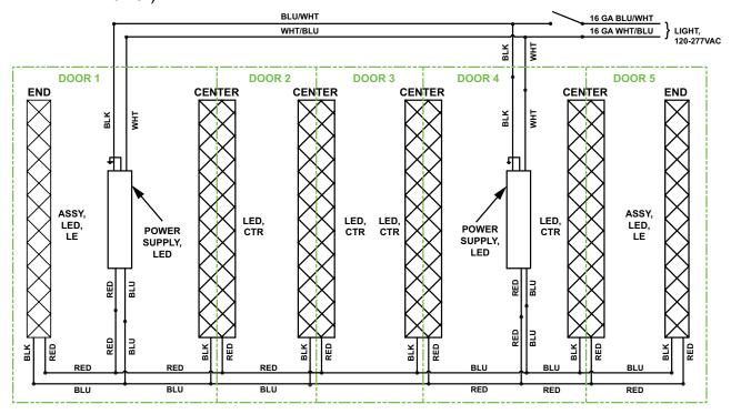
Model 401 Optimax Pro 24V Wiring Diagram (6-Door: 48" & 54" Low Power)
