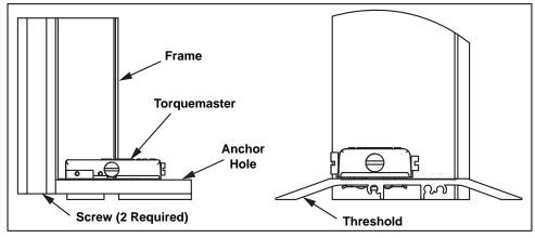
Pass-Thru Cross-Section (with/without Threshold)
