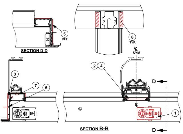
Model 401 Frame Section B Replaceable Parts
