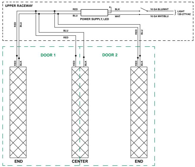
Model 401 Wiring Diagram (07-21941-0002), 2-Door
