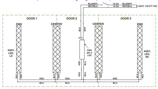
4. Model 401 Optimax Pro 24V Wiring Diagram (4-Door)
