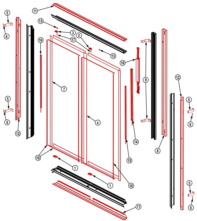
Model 401 Frame Exploded Diagram
