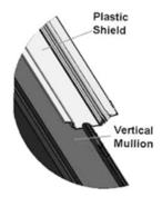
c. Using a Phillips screw driver, thread a #8 tapping screw through the plastic extrusion.
