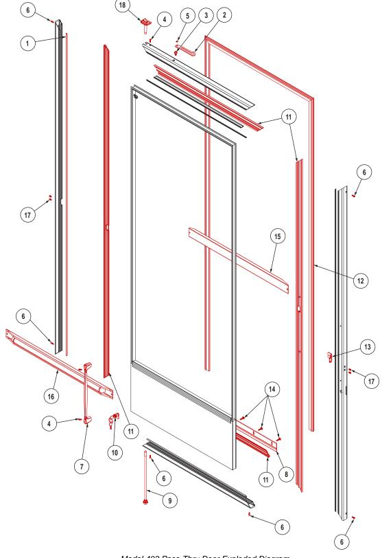
Model 403 Pass-Thru Door Exploded Diagram
