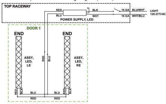
2. Model 401 Optimax Pro 24V Wiring Diagram (2-Door)
