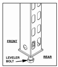
3. Insert front of shelf into front post at angle, then position rear shelf posts.
