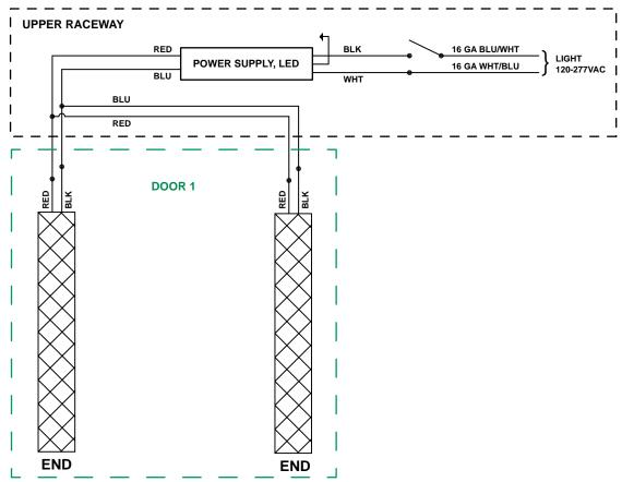
Model 401 Wiring Diagram (07-21941-0001), 1-Door
