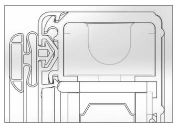
2. To replace, start at bottom of door. Insert gasket into groove in both sides of door and slide gasket up to top of door. Tuck in all four corners with flat-head screwdriver.
