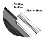
f. Using a Phillips screw driver, thread a #8 tapping screw through the plastic extrusion.
