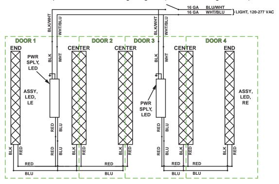
6. Model 401 Optimax Pro 24V Wiring Diagram (5-Door: 48" High Power & All Low Power)
