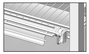
2. Snap top corner of tag molding strip onto shelf front. Apply even pressure across top of tag molding as it is fed onto top horizontal bar on shelf front.
