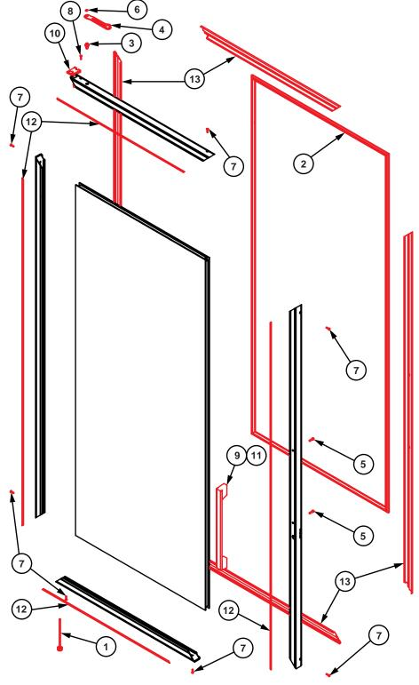
Model 401 Door Exploded Diagram
