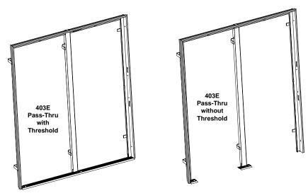
2. When no threshold is desired, drill and lag on pre-drilled mounting holes only.
